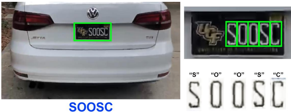
Figure 2.1: Example of License Plate Detection Using Computer Vision
