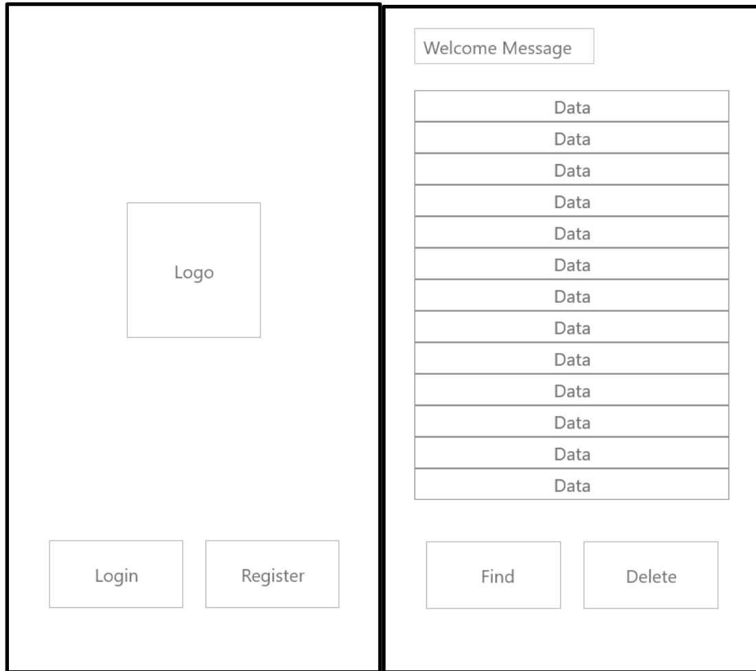
Figure 5.10: Mobile Application Component Wireframe
